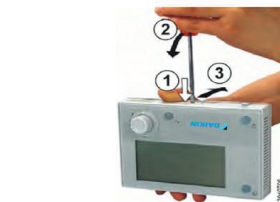
Cover Removal: through the wall wiring connection
