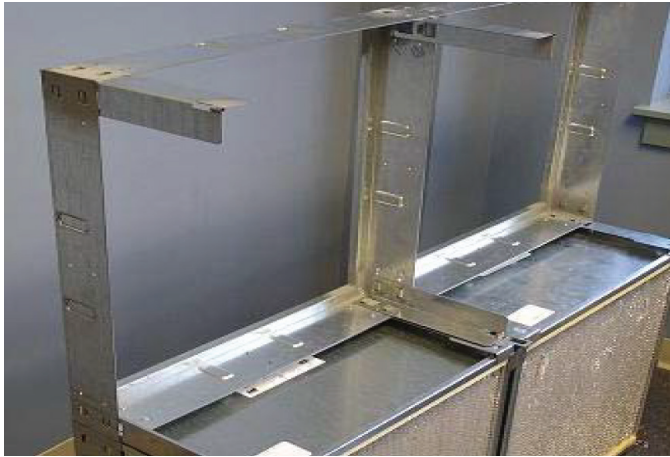
Figure 99: Frame with Leg Extensions Installed
